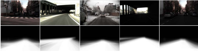
Fig. 5. Example results of online road prior generation. Given (top row) a georeferenced image, a confidence map with the per-pixel potential of being a road pixel is generated based on (bottom row) digital road maps and GPS information. The algorithm does not depend on image features, and thus, the confidence map is recovered despite lighting variations or imaging conditions. Additional results can be found at http://www.josemalvarez.net .
