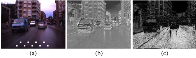
Fig. 6. Color cue from a single image. (a) Input image with seeds used to estimate the road model p(\cdot) . (b) Shadow-free image \mathcal{I} . (c) Road confidence map depicting the potential of a pixel being a road pixel. The whiter the color, the higher the potential.
