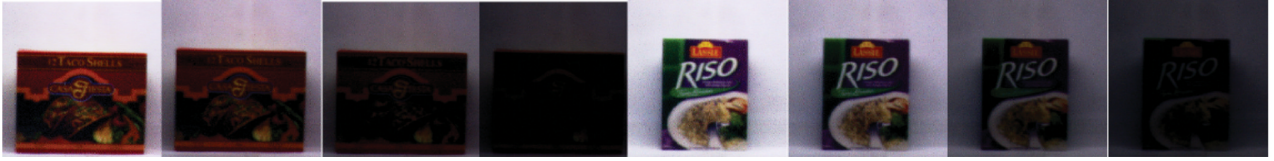
Fig. 5. Two objects under varying illumination intensity generating each four images with \text{SNR} \in \{24, 12, 6, 3\} . (Color version available online at http://ieeexplore.ieee.org .)
