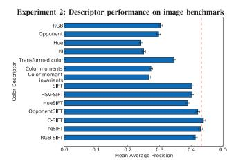
Fig. 6. Evaluation of color descriptors on an image benchmark, the PASCAL VOC Challenge 2007 [21], averaged over the 20 object categories. Error bars indicate the standard deviation in mean average precision, obtained using bootstrap. The dashed lines indicate the lower bound of the C-SIFT confidence interval.
