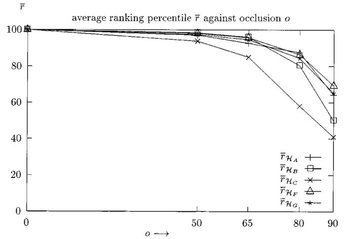
Fig. 11. Ranking percentile plotted against the percentage object area blanked out  $o$  denoted by  $\bar{r}_{\mathcal{H}_A}$ ,  $\bar{r}_{\mathcal{H}_B}$ ,  $\bar{r}_{\mathcal{H}_C}$ ,  $\bar{r}_{\mathcal{H}_F}$ , and  $\bar{r}_{\mathcal{H}_G}$ .
