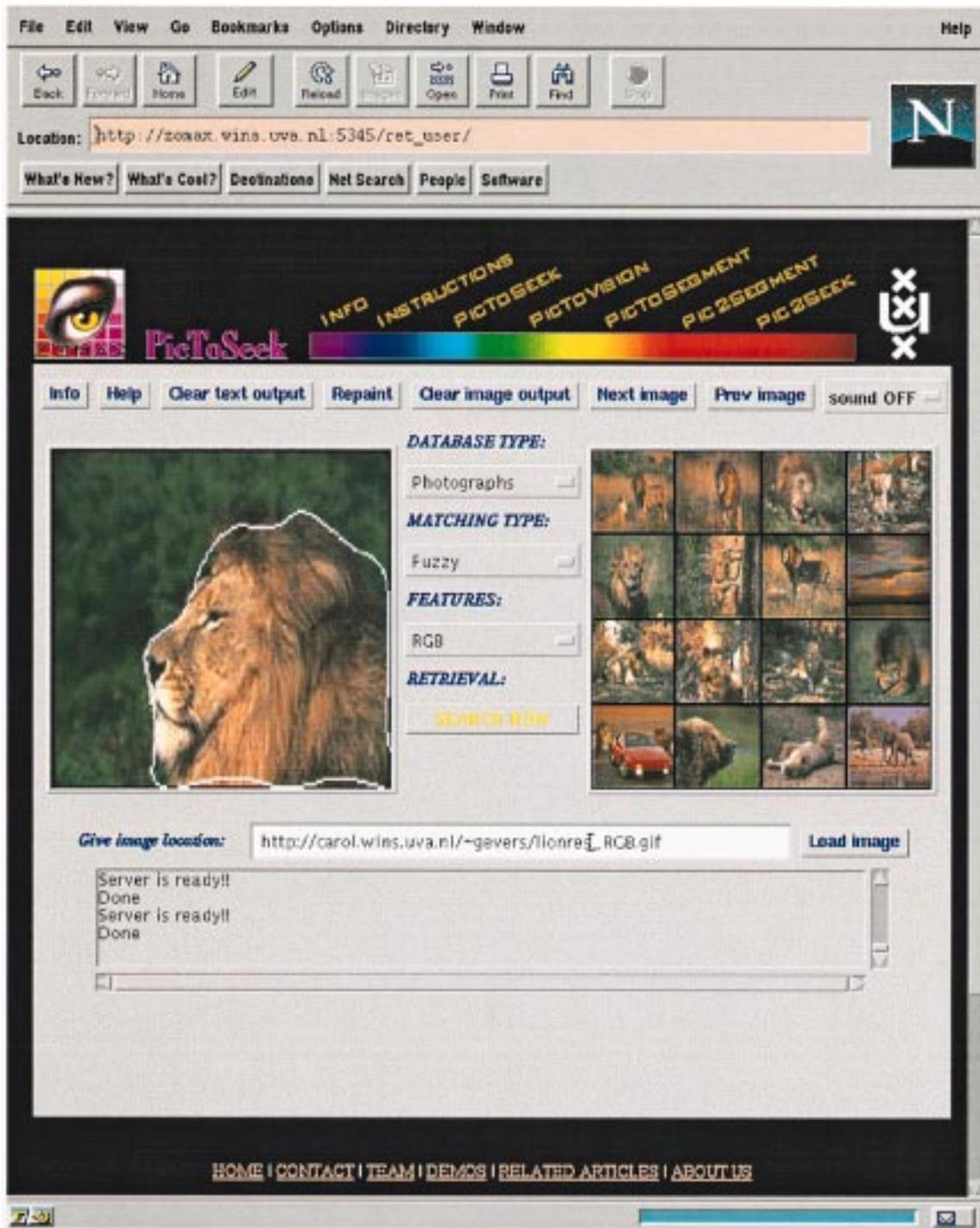
Fig. 14. Content-based image retrieval by query-by-example based on the region denoting the lion (without the background) as specified by the user.
