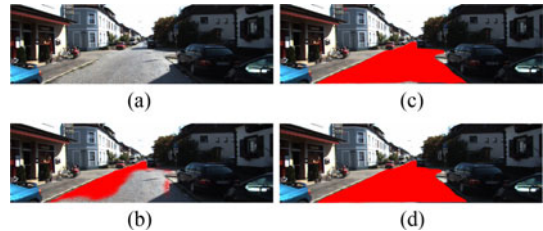
Fig. 1. Different textures on road appearances between training and testing sets can lead to false segmentation. (a) Input image. (b) Result of a fully supervised segmentation network. (c) and (d) Results of our SSL and WSL methods. The predicted road areas are denoted in red.
