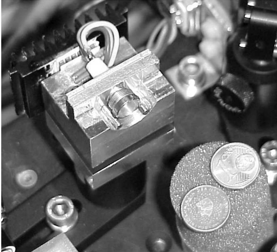
Figure B.3: *photograph of the lasermount. The euro-cent coils are to indicate the scale.*
