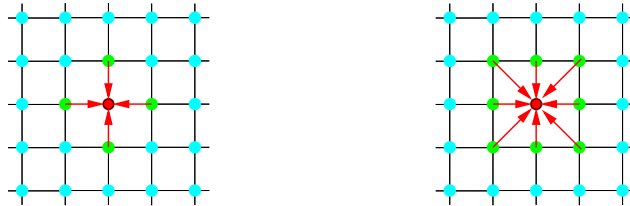
Fig. 23. Algorithmic principle of convolution, shown is the 2-dimensional case with a 5-point stencil (left) and a 9-point stencil (right)
