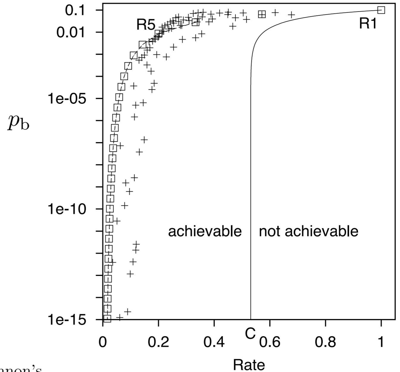
Figure 1.19. Shannon's noisy-channel coding theorem. The solid curve shows the Shannon limit on achievable values of  $(R, p_b)$  for the binary symmetric channel with  $f = 0.1$ . Rates up to  $R = C$  are achievable with arbitrarily small  $p_b$ . The points show the performance of some textbook codes, as in figure 1.18.
