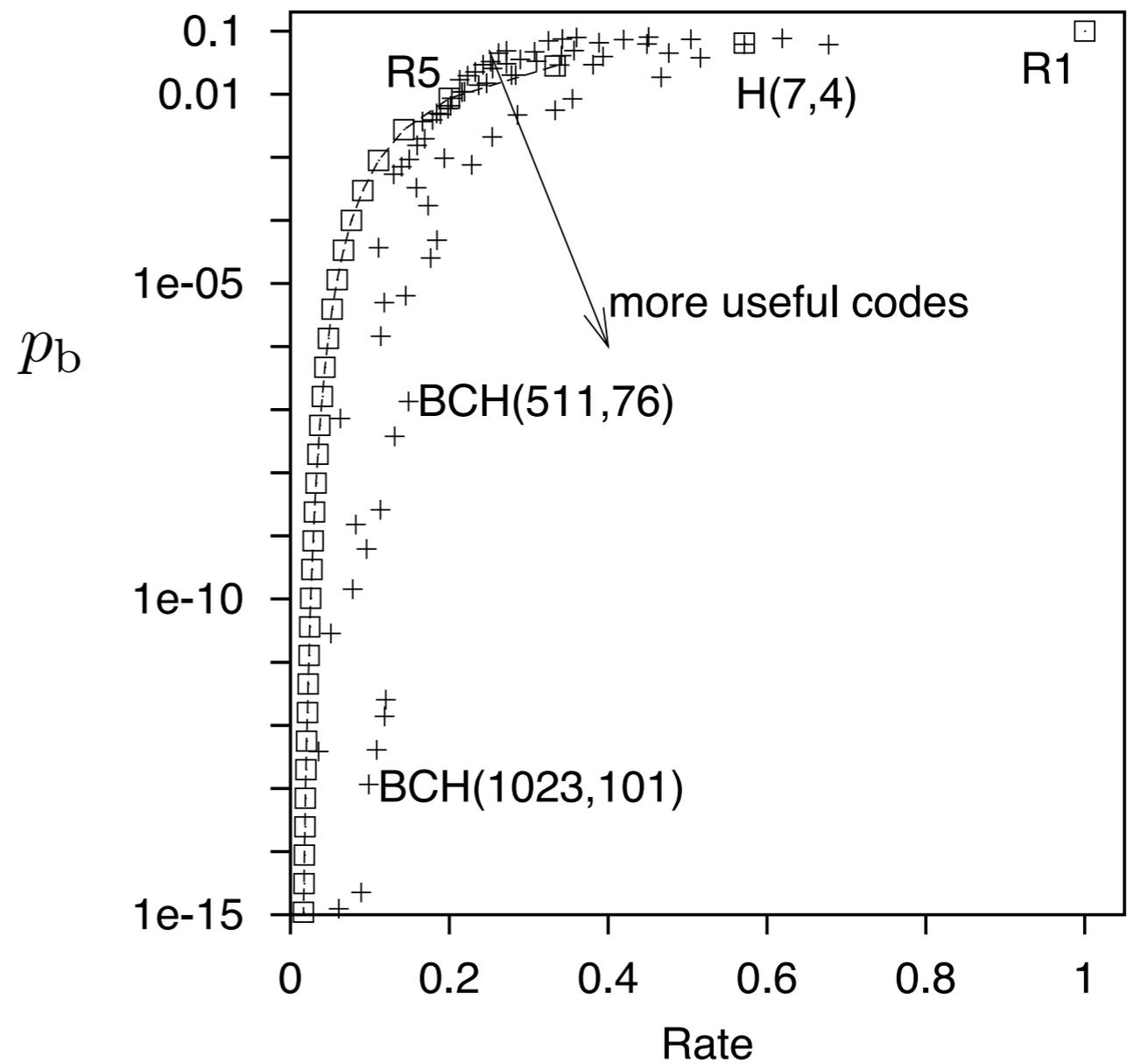
Figure 1.18. Error probability  $p_b$  versus rate  $R$  for repetition codes, the (7,4) Hamming code and BCH codes with blocklengths up to 1023 over a binary symmetric channel with  $f = 0.1$ . The righthand figure shows  $p_b$  on a logarithmic scale.
