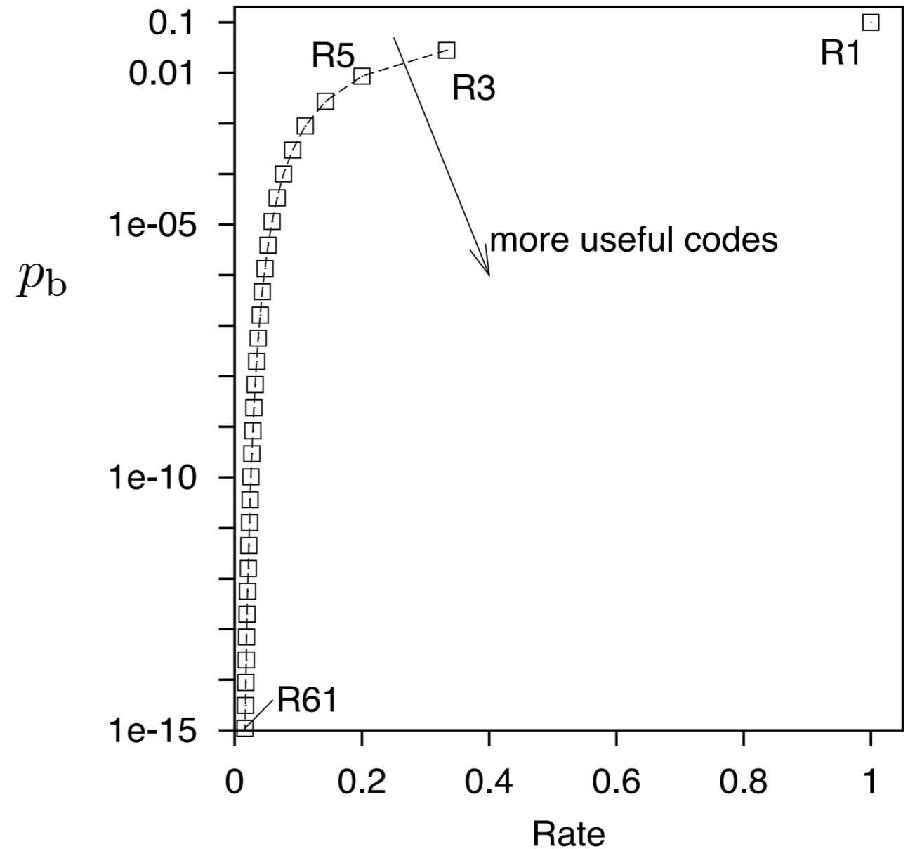
Figure 1.12. Error probability  $p_b$  versus rate for repetition codes over a binary symmetric channel with  $f = 0.1$ . The right-hand figure shows  $p_b$  on a logarithmic scale. We would like the rate to be large and  $p_b$  to be small.
