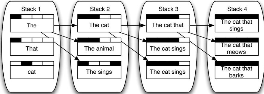
Figure 2.2: A trivial example of the stack based decoding framework used in this thesis, given the French sentence to translate “Le chat qui chant.” We display bit vectors above the different states in the translation stacks.
