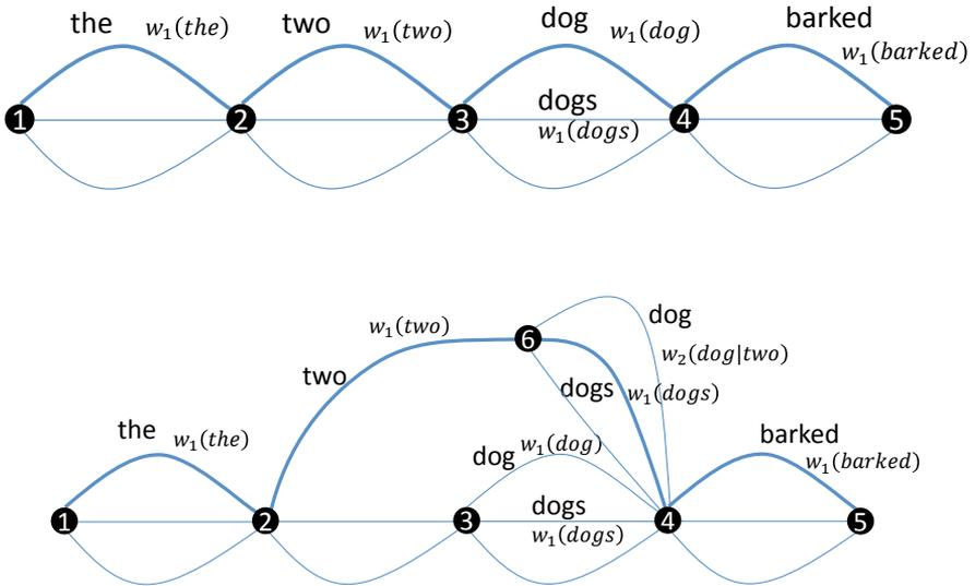
Figure 7.1: An example of an initial  $q$ -automaton (a), and the refined  $q$ -automaton (b) Each state corresponds to a context (only state 6 has a non-empty context) and each edge represents the emission of a symbol. Thick edges are representing the path for the sampling/decoding of `two dog(s) barked`, thin edges corresponding to alternative symbols. By construction,  $w_1(dog) \geq w_2(dog|two)$  so that the total weight of (b) is smaller than the total weight of (a).
