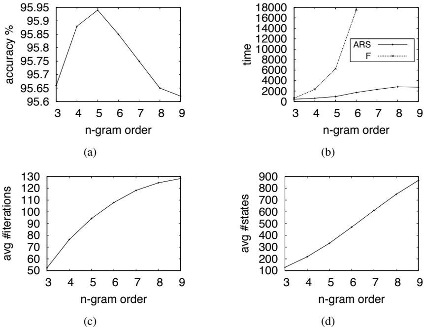
Figure 7.4: In 7.4a, we report the accuracy results given different  $n$ -gram models on the WSJ test set. In 7.4b, we show the time taken (seconds) to decode the WSJ test set given our method (ARS), and compare this to the full model (F). In 7.4c, the average number of iterations needed to sample the test set given different  $n$ -gram language models is given, and 7.4d shows the average number of states in the variable-order HMMs.
