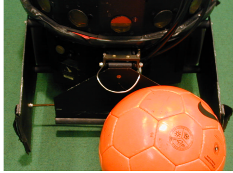
Figure 2.4: The kicker, ball handlers and the ball handling mechanism.
