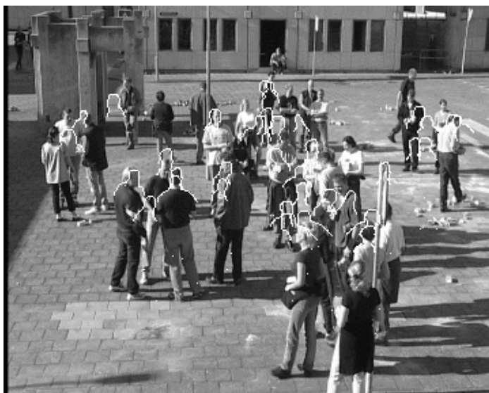
(c) Shape-based detection with ground plane constraint and person/non-person classifier
