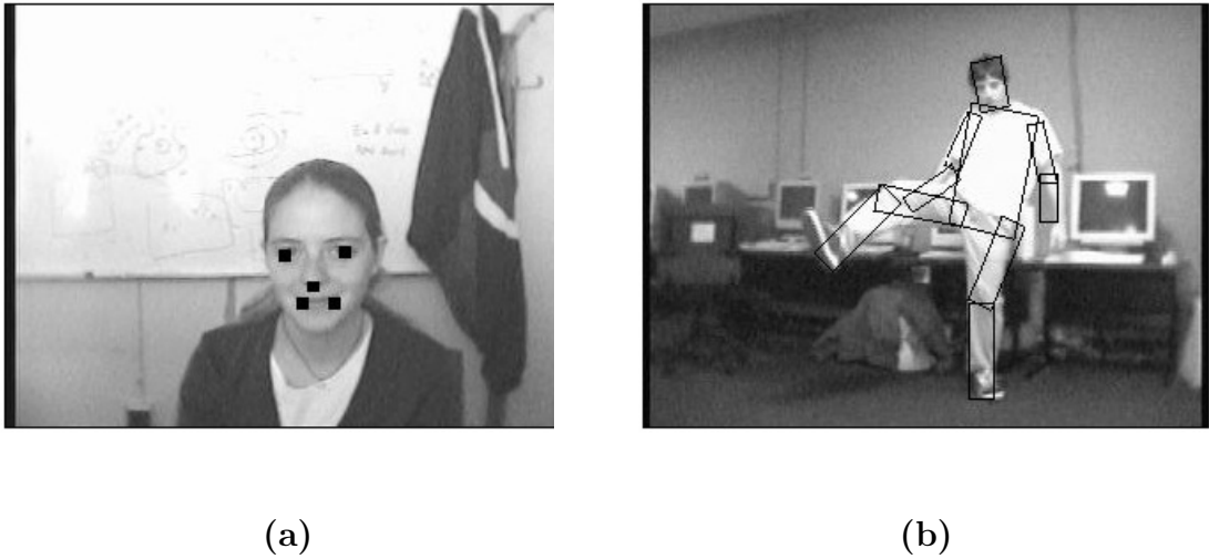
Figure 2.1: Examples of two pictorial structure models matched against images. (a) detection of a face; (b) detection of a human body. Adapted from [8].
