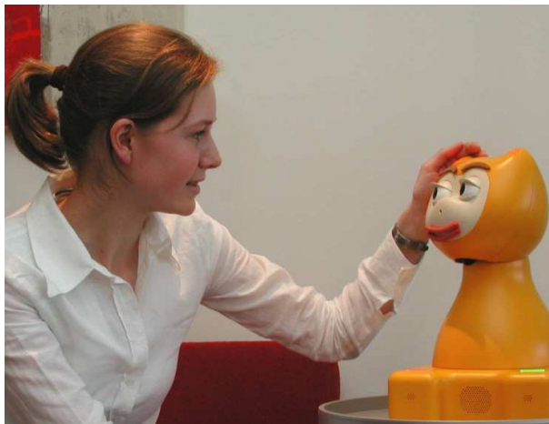
Figure 1.1: Philips iCat interface robot. The two microphones are mounted on the sides of the bottom panel.
