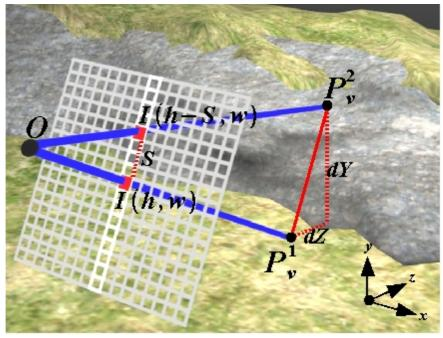
Figure 2.18: Columns based slope estimation.
