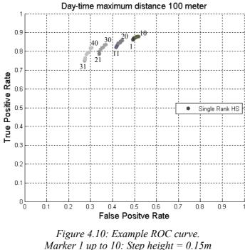
Marker 1 up to 10: Step height = 0.15m Marker 11 up to 20: Step height = 0.30m Marker 21 up to 30: Step height = 0.45m Marker 31 up to 40: Step height = 0.60m For the ten markers in each set the hysteresis threshold values can be found in table 4.2.
