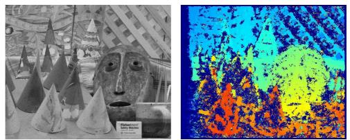
Figure 4.6: Original with noise (left), Unfiltered disparity estimate (right).
