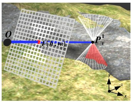
*Figure 2.23: Truncated cones approach. Truncated cones are projected to two triangles in the image. red terrain is compatible with*  $P_v^1$ .
