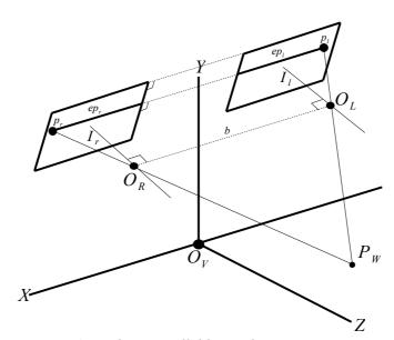
Figure 2.4: Photo parallel binocular camera system.
