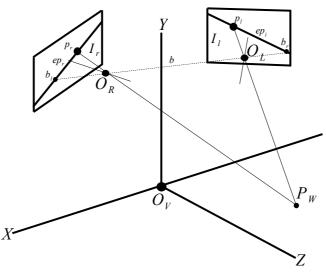
Figure 2.5: Non rectified binocular camera system.
