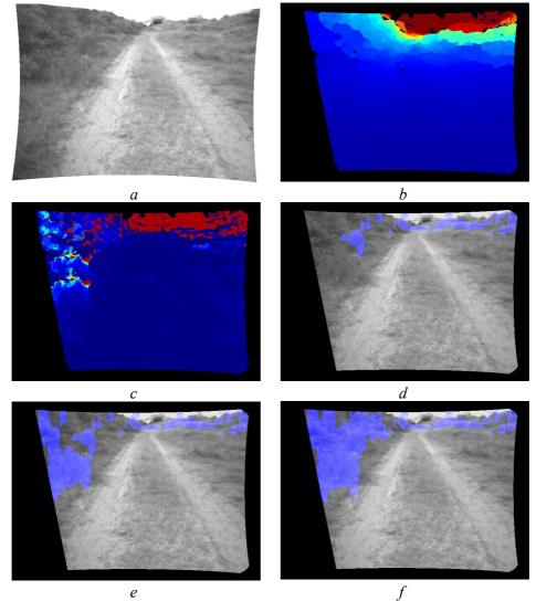
Figure 4.14: Original image (a), computed depth map (b), computed slope map(c), Regular threshold 0.75 (d), hysteresis thresholding [0.5 0.75] (e) and [0.25 0.75] (f).
