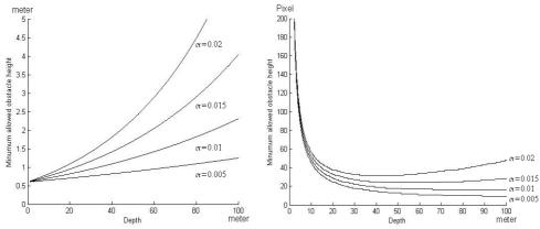
Figure 3.8: Depth dependent height threshold in meters (left) and pixels (right).
