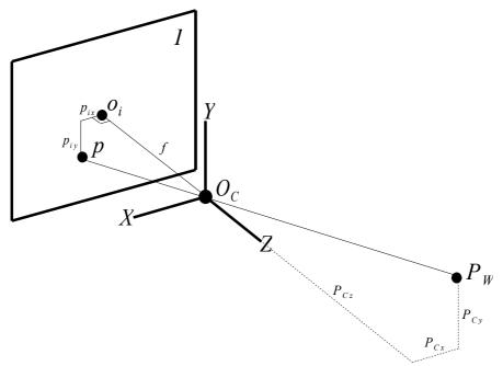
Figure 2.2: Pin-hole camera model.
