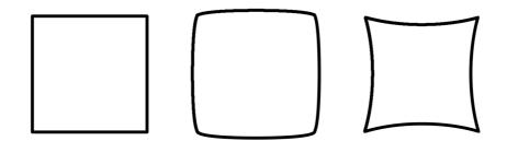
Figure 2.3: Effects of radial distortion, undistorted (left), barrel distortion (middle), pincushion distortion(right).
