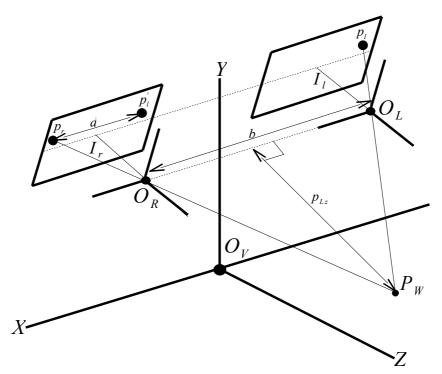
Figure 2.1: Binocular camera model.
