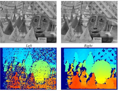
Small aggregation windowLarge aggregation windowFigure 2.11: Effect of aggregation window size.
