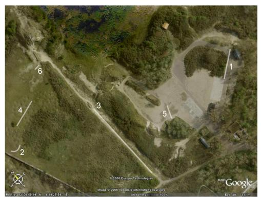
*Figure 3.10: Test terrain, 1 big gap 2 concrete wall, 3 Rock pile, 4 Holes, 5 Sand plane, 6 Trunks.*
