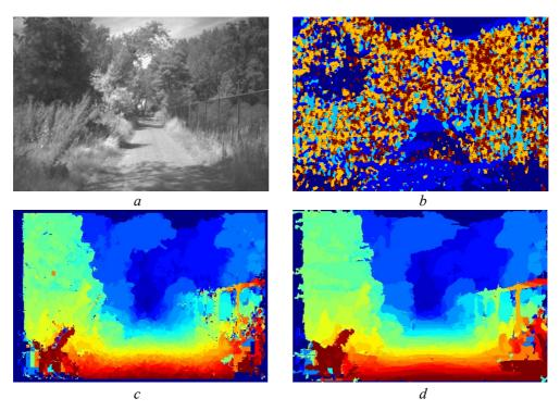
Figure 6.1: Using texture segmentation to improve disparity estimate. Left image of stereo image pair (a) and its texture segmentation (b), disparity map (c), texture enhanced disparity map (d).
