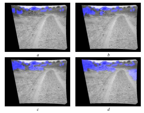
Figure 4.13: Effect of hysteresis thresholding, 0.75-0.75(a) 0.75-0.25(b) 0.75-0.15(c) 0.75-0.05(d).
