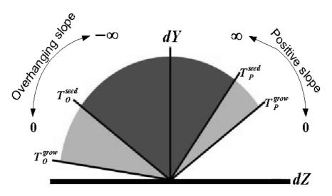
Figure 3.7: Hysteresis based thresholding
