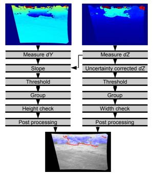
Figure 3.3: Obstacle detection system overview, positive obstacles left column, negative obstacles right column.
