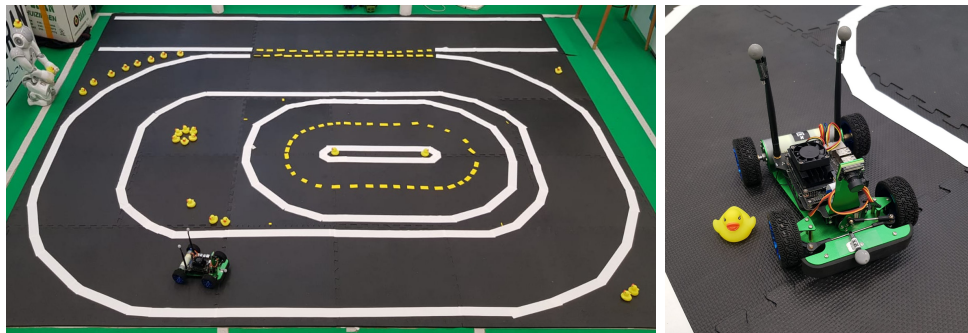
Figure 3.2: The DuckieTown highway used for real world evaluation. The outer track circle is used for the JetRacer. The JetRacer vehicle is shown at the right.
