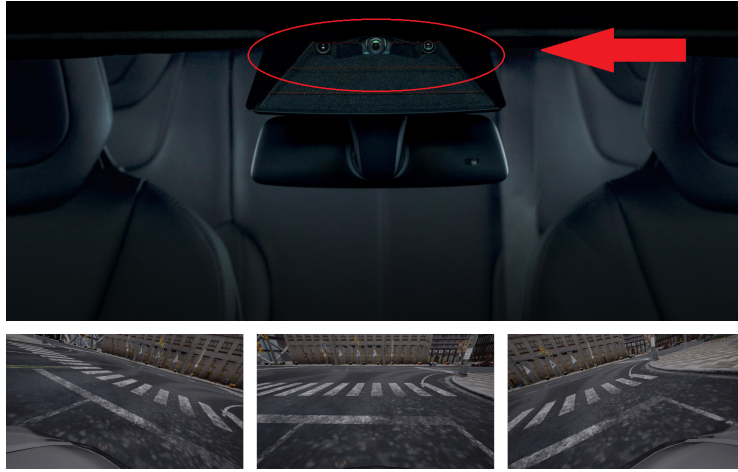
Fig. 2: Example of triple-cam setup behind car’s windshield, with below this example the view of the triple camera’s from left, middle to right camera.
