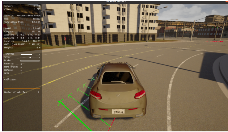
Fig. 3: CARLA simulator with model inference vector (green) and vehicle forward vector (red).
