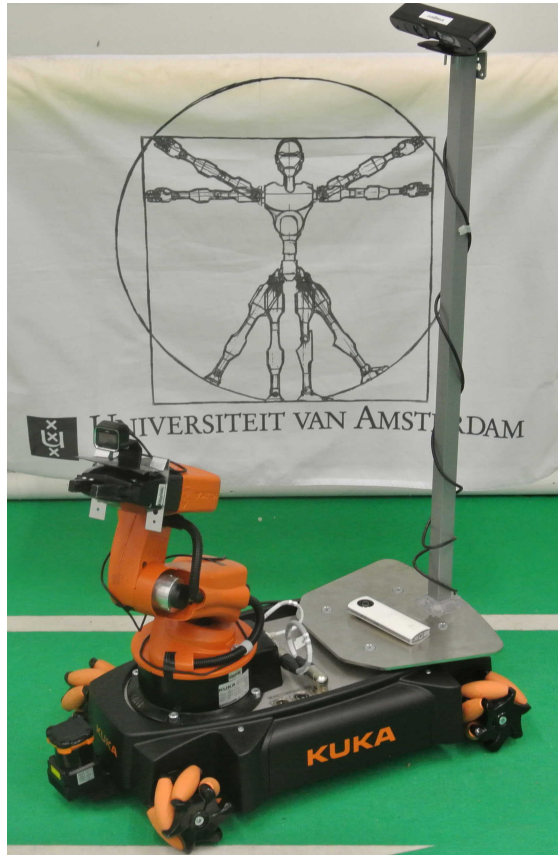
Figure 1: The Kuka youBot mounted with all its sensors: Asus Xtion Pro Live, Hokuyo UTM-30LX and a Microsoft LifeCam HD-5000.
