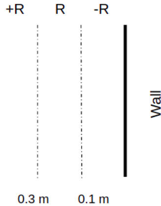
Figure 6: Visualization of the wall distance. R corresponds to being in the perfect distance to the wall, -R is close to the wall and +R to far.
