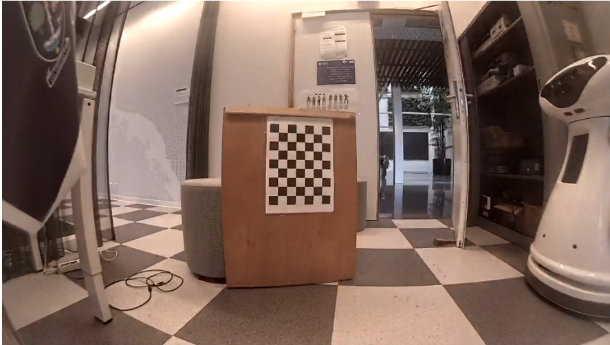
Figure 5: Distorted image before calibration
