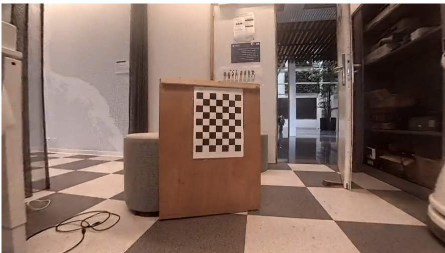
Figure 6: Undistorted image after calibration
