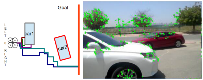
Figure 9: The path of the AR.Drone avoiding two cars (left), based on the processed image (right)
