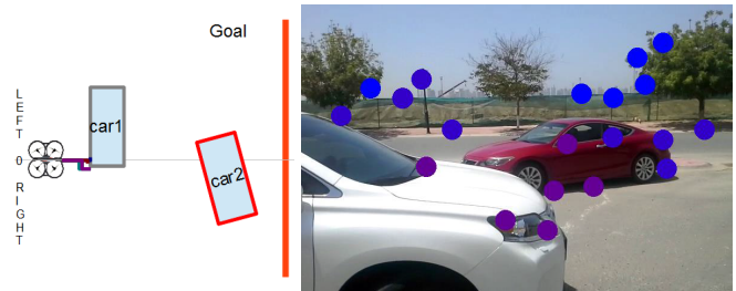
Figure 10: The path of the AR.Drone between two obstacles, without depth classification
