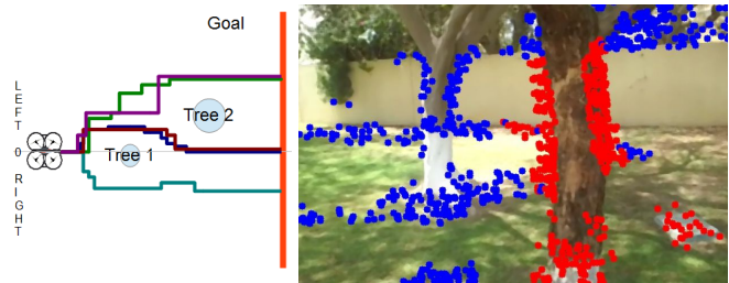
Figure 3: The path of the AR.Drone between two obstacles (left), based on the image including depth classification (right)
