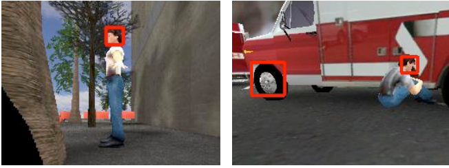
Fig. 1. Our face detector can recognise faces at greater distances than the VictimSensor. Some detections are false positives, but these can be used as negative examples in subsequent levels of training.
