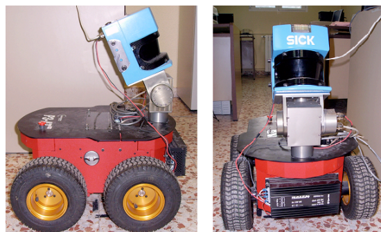
Fig. 1. Left:3D data acquisition system, mounted on our robot Nemo.
