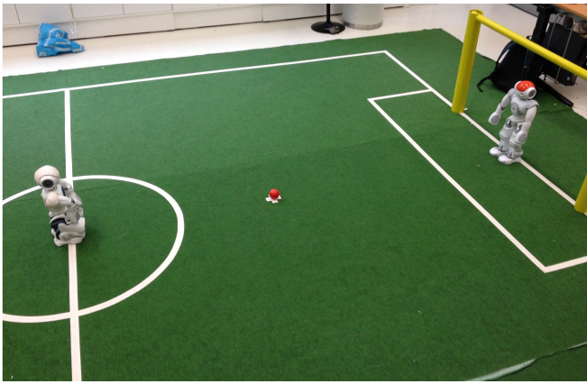
Fig. 5: Typical start of a penalty shootout. The opposing player (left) starts at the center line, with a distance of 3 meters from the goal, walks towards the ball and kicks it. The goalkeeper starts at the goalline.
