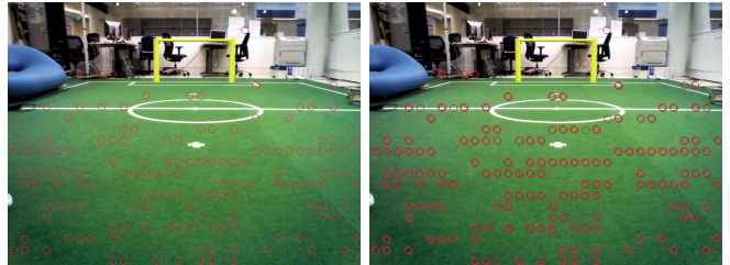
Fig. 6: Two consecutive timesteps of a noisy motif z for N_z = 5 , T_z = 10 . Circles indicate cells where optical flow is detected, with the thickness of the circle corresponding to presence p(w|z) . As optical flow is detected throughout almost the entire image, this motif is too general to be of use.
