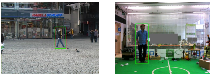
Fig. 2. People detection by CNN examples. Left: Training on TUD-Motionpairs, Right: Verification in lab (IRL dataset)
