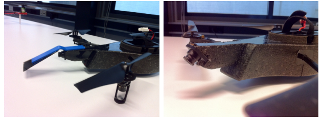
Figure 3. Possible solutions to solve the camera configuration problem, the mirror construction (left) and the modification of the AR.Drone (right)
