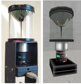
Fig. 1. The catadioptric omnidirectional camera, real and simulated.
