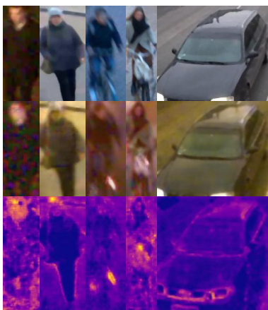
Fig. 4: Examples of AU-GAN’s input imagery (top), i.e. imagery from FlowCube’s re-id training dataset, their respective AU-GAN transformed nighttime equivalent (middle), and the corresponding confidence maps (bottom).
