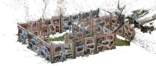
Fig. 11. A dense 3D reconstruction of the mini maze with COLMAP. Courtesy den Braber et al.
