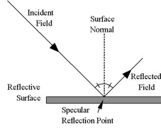
Fig. 7. Specular reflection is used in ray tracing
