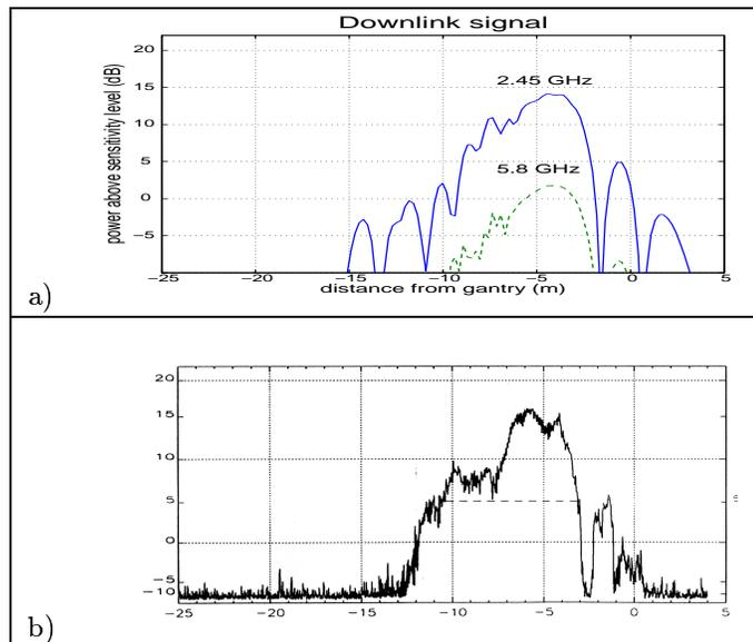
Fig. 9. Calculation and measurement of the received power at  $Y=0$  and  $\theta_{OBU} = 45^\circ$  for a vehicle with a bonnet driving next to a large truck. The measurement is taken from [4, page A.25].
