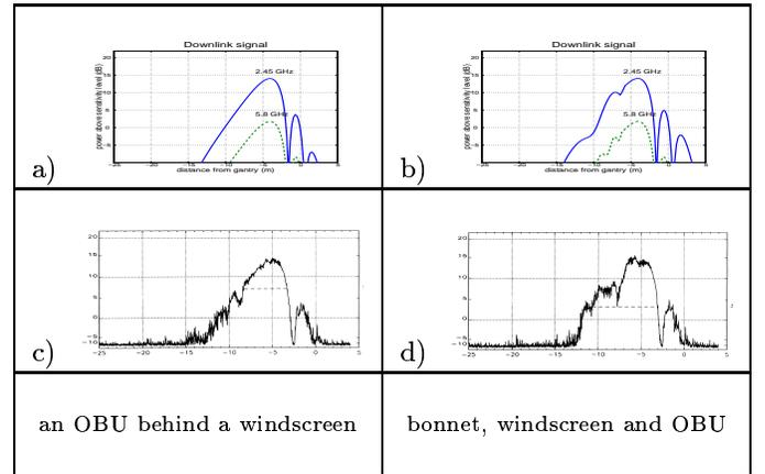
Fig. 8. Calculations and measurements of the received power at  $Y=0$  and  $\theta_{OBU} = 45^\circ$  for a vehicle with and without a bonnet. The measurements are taken from [4, page A.16 & A.17].
