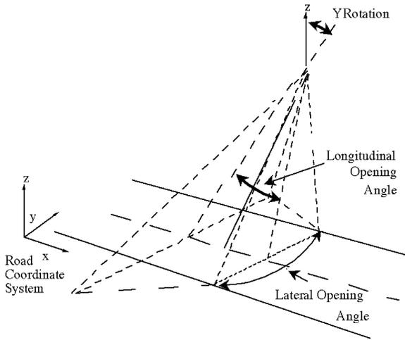
Fig. 1. Definition of a VolumeTriangle
