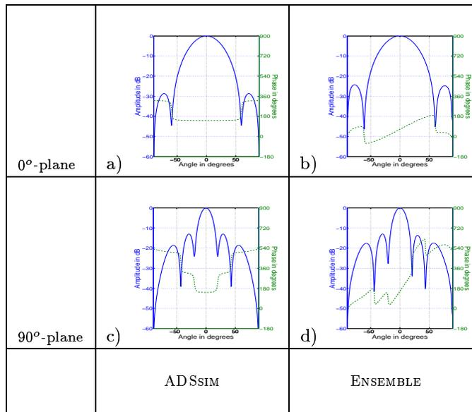
Fig. 11. Array antennas field patterns obtained with our Transmitter Field Single Receiver Model (a,c) and ENSEMBLE (b,d) for two planes through the z-axis. Both programs used a 4 by 2 array antenna with circularly polarised square patches with length of 2.65cm, substrate thickness of 0.265cm, operating frequency of 5.8GHz and dielectric constant of 1. (Solid line: amplitude, dashed line: phase.)
