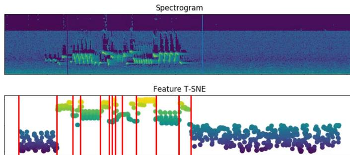
Fig. 5: t-SNE of CNN features covarying with phrases
