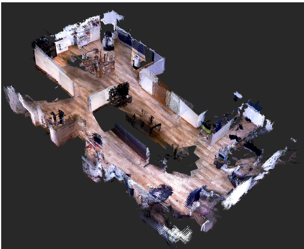
Figure 7.2: 3D pointcloud viewer of a single trajectory through the environment.
