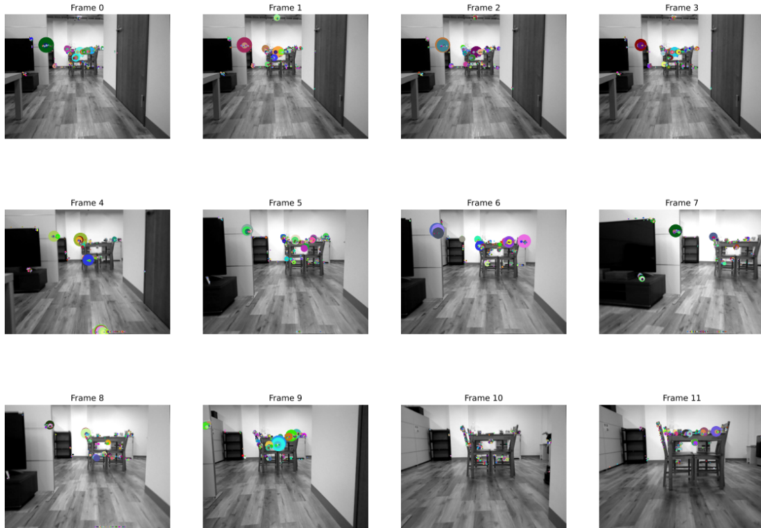
Figure 7.6: The found keypoints using the R2D2 feature detector. Note that the larger the circle is, the more confident the detector is.
