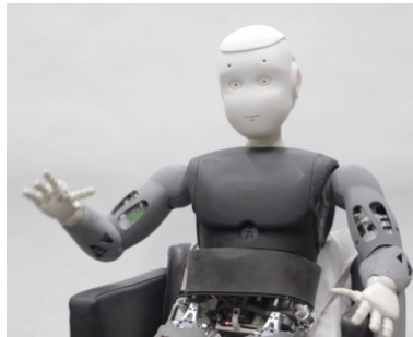
Figure 1.1: Romeo is a prototype under development, designed to assist people at home.
