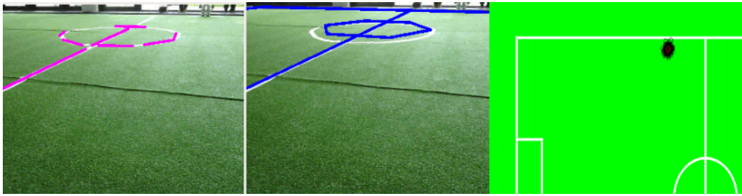
Figure 2.4: Example of the localisation method that relies on detecting lines. In the left image, the white pixels are detected. In the centre image, a line model is formed based upon the detected pixels. In the right image, a particle filter determines the most likely position on the football field.
