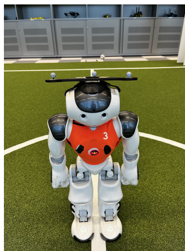
Figure 3.9: 3D printed Optitrack helmet on the Nao V6 robot.
