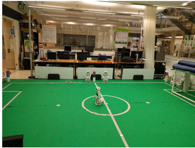
Figure 1: The field of the RoboCup Soccer as used in the experiment. The Nao robot will walk several times the 8-shaped path marked on the field.
