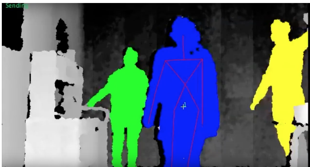
Figure 8: During the steps, other users are recognized but not tracked.
