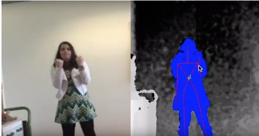
Figure 7: The joints of the user are detected as a skeleton.
