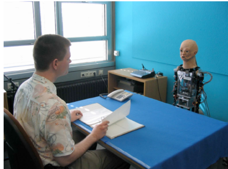
University of Bielefeld: Anthropomorphic robot BARTHOC Jr. Robot recognizes emotional content (happiness, fear and neutral) from speech and mirrors it by facial expressions.
