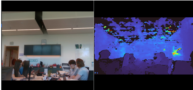
Figure 12: Rerun visualization of image (left) and depth image (right)
