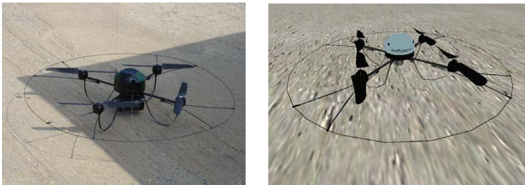
Figure 1: The AirRobot is a four-rotor electrical helicopter with flight stabilization control produced by AirRobot Co. Left a real robot, right a simulated version.
