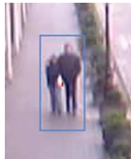
Figure 8 the people in the frame are detected as a moving region at low speed
