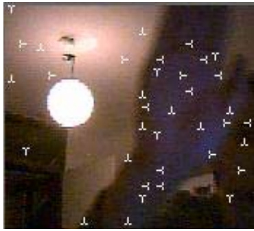
Figure 6a – optical flow with arrows
