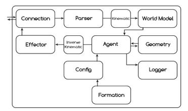
Fig. 1 . Scorpius Agent Architecture: Connection unit connects agent to the server, and passes data form server to the parser unit. Then WorldModel will be updated using these data. Also in order to obtain coordinates of each body section such as hands, legs and torso, it uses Kinematic unit. The agent makes a decision using WorldModel data, formation and geometry tools and sends it to the server by using some classes such as Effector and Connection.
