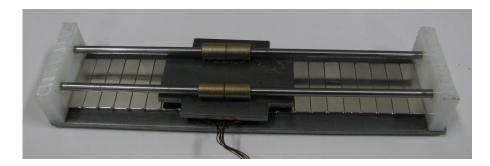
Fig. 3. Linear motor kicker prototype.
