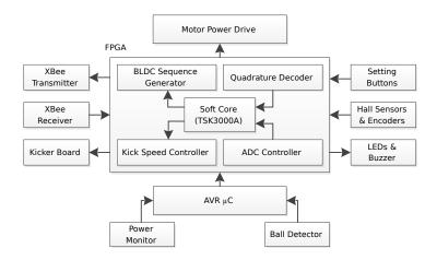
Fig. 7. The electrical system's diagram
