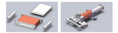
Fig. 5. (a) The new chip kick solenoid and plunger (b) The new linear kick solenoid and plunger
