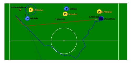
Fig. 2. The generated path before and after smoothing
