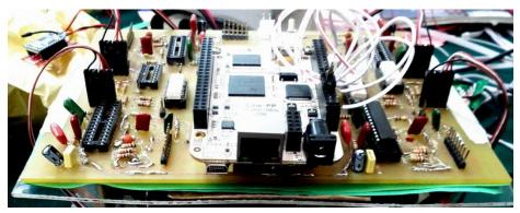
Fig 2.1 BeagleBone and its peripheral circuitry
