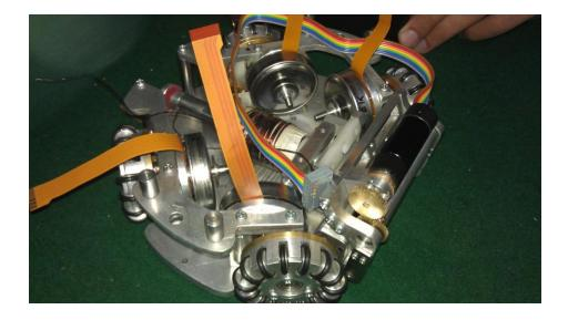
Fig 3.3 Complete Assembly with Dribbler Mechanism
