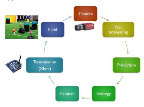
Fig 4.1 Software System Architecture
