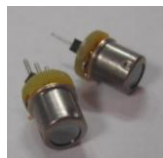
Fig. 5. RKRS custom thermal sensors with Perkin Elmer thermopile elements.
