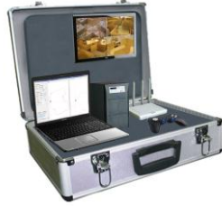
Fig. 1. Aluminum wheeled case to be used to carry all necessary items for the operator station.
