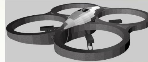
AR.Drone (including camera and sonar)
