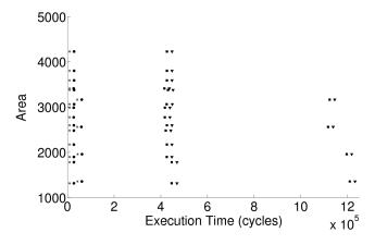
Fig. 6. Pareto plot representing the latency values included in the *calibration table* annotated with the area value corresponding to the related ASIP configurations. Different symbols are used to represent values associated to different tasks in the M-JPEG kernel
