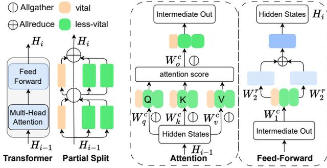
Fig. 3: Transformer Partitioning
