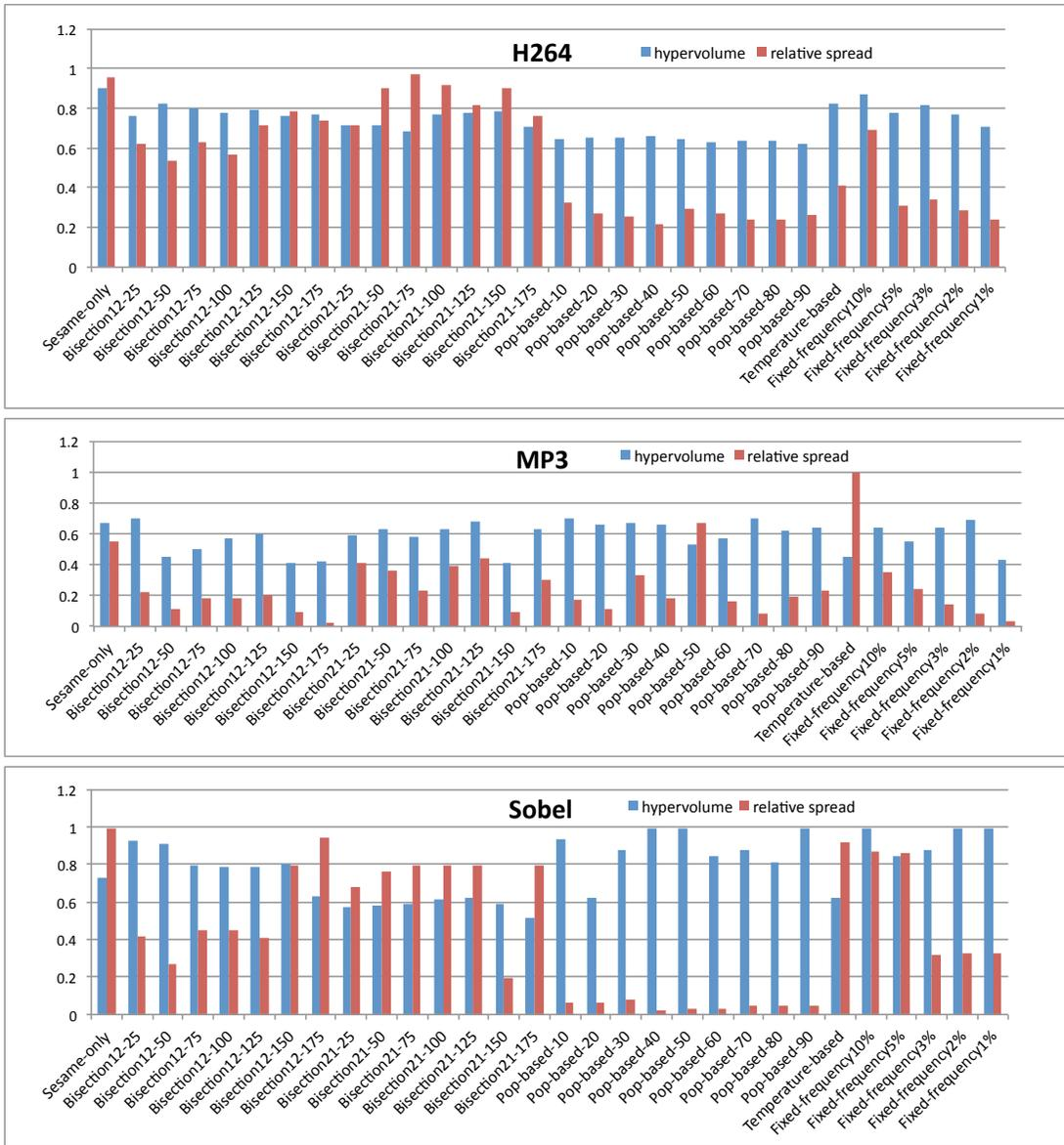
Fig. 6. Average hypervolume and  $\nabla$  values for the different DSE methods applied to the Mp3 decoder, H264 decoder, and Sobel filter applications.
